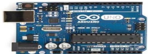
Figure1: Arduino UNO Board
